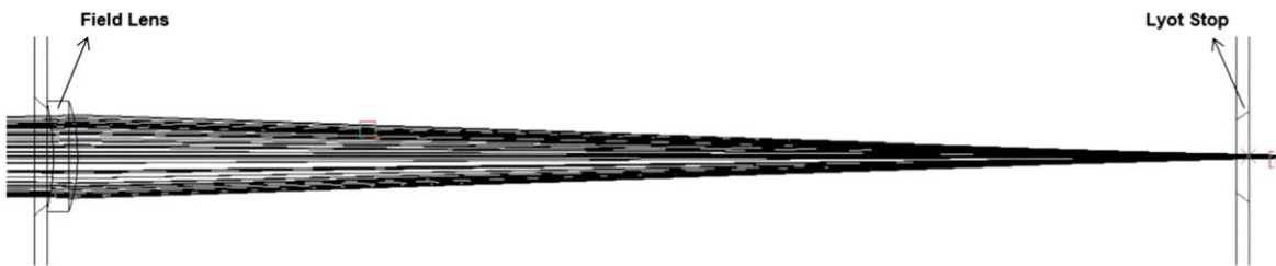
Figure 4. The secondary reflected light of the objective lens is refocused by the field lens at the Lyot stop.
